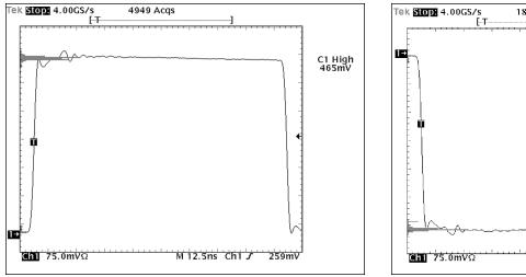
Figure 8. Positive MLT-3 pulse with high automatic measurement.
