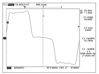
Figure 6. Duty cycle distortion measurement, positive pulse width.
