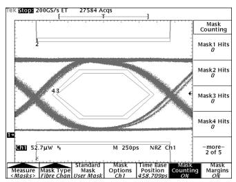
Figure 12. Eye diagram masks with 20% margin added.
