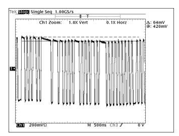
Figure 2. Baseline wander in a 100Base-TX frame at higher resolution.
