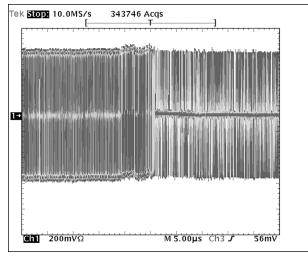
Figure 1. Baseline wander in a 100Base-TX signal observed with DPO.
