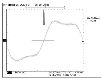
Figure 10. Random jitter measurement.
