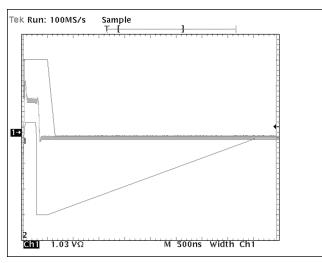
Figure 3. 10BaseT idle pulse mask.
