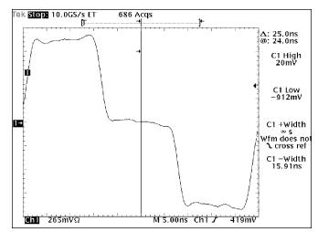
Figure 7. Duty cycle distortion measurement, negative pulse width.
